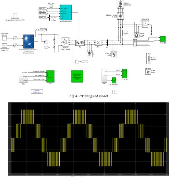
(a) Unfiltered Inverter output voltage
