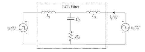
Fig.2: L-C-L filter and components [2]
